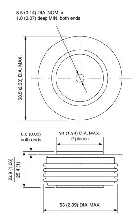
Quote between upper and lower pole pieces has to be considered after application of mounting force (see Thermal and Mechanical Specifications)
